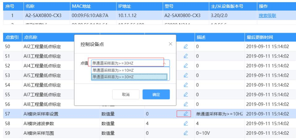
The screenshot shows a software interface for managing device parameters. At the top is a table with columns: 序号 (Index), 名称 (Name), MAC地址 (MAC Address), IP地址 (IP Address), 型号 (Model), 主/从设备版本号 (Master/Slave Device Version Number), and 操作 (Operation). One row is selected, showing index 1, name A2-SAX0800-CX3, MAC address 00:09:F6:10:A8:7A, IP address 10.1.1.12, model A2-SAX0800-CX3, version 3.20/2.0, and operation '搜索级联' (Search Cascading).
